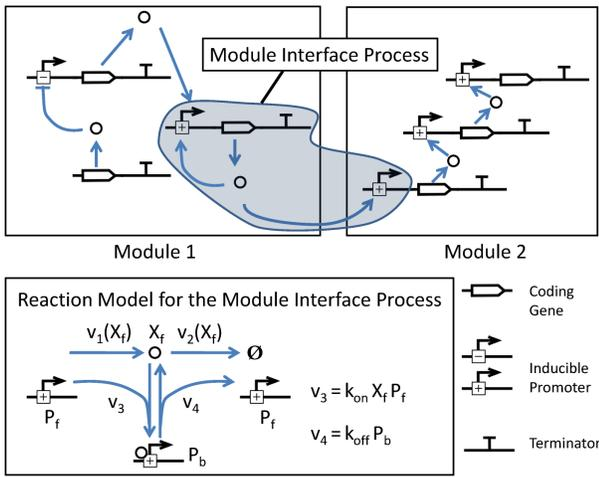
Fig. 1: Module interface process between Modules 1 and 2
